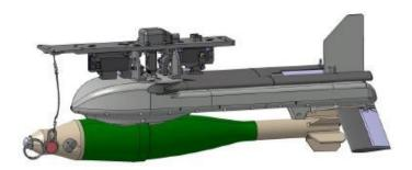
Gliding guidance kit is meant for conversion of existing 60 mm mortar rounds into an affordable guided munition. Because of its small mass and dimensions, it can be carried by numerous UAVs. After release, wings on the guidance kit open providing greater range. This weapon enables high precision attacks on enemy infantry. Guidance is completely autonomous relying on GPS/INS. The system enables attacks both on fixed coordinates or on the coordinates provided by the EO payload on the UAV.
