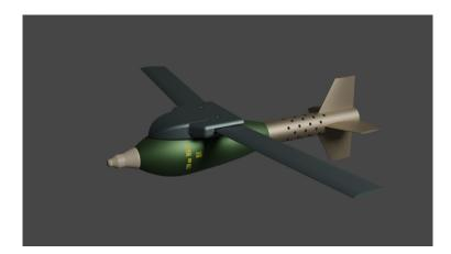
Gliding guidance kit is meant for conversion of existing 120 mm mortar rounds into an affordable guided munition. Because of its construction, it can be carried by numerous UAVs. After release, wings on the guidance kit open providing greater range. This weapon enables high precision attacks on enemy infantry. Guidance is completely autonomous relying on GPS/INS. The system enables attacks both on fixed coordinates or on the coordinates provided by the EO payload on the UAV.
