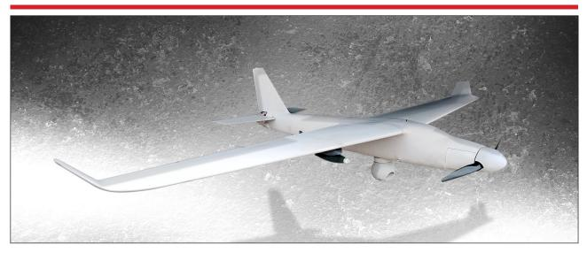
Short range armed UAV "Senka", designed for day and night reconnaissance and surveillance, and destruction of light targets. With catapult launch and parachute landing it enables airfields free operations. The UAV features fully autonomous guidance and can be armed with 12 light 40 mm grenades or two 60 mm glide kits for attacks from distance. Operational package consists of: UAVs, Ground Control Station, Remote Video Terminal, Weapons, Catapult, transport equipment and set of tools.
