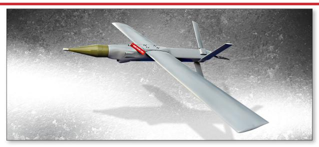
Loitering munition OSICA is a fully autonomous loitering unmanned aerial system designed for attack missions (KAMIKAZE). It is a cost-effective high-precision loitering munition with capability to destroy armored vehicle. UAS is equiped with shaped-charge warhead from anti-tank weapon system M79 Osa. With fixed ultra compact Full-HD camera modul and video processor it is able to detect and fully autonomously attack target based on video tracking system.
