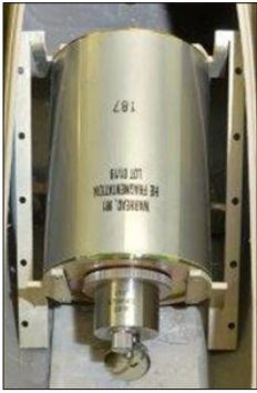
Combined (blast & fragmented), with steel balls, 130mm, total mass 10.5 kg
