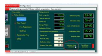
Artillery fire control system (AFCS) supports ballistic computation for different calibers (including 155 mm). Rugged hand-held computer model Algiz 10x is used for application software for FCS.
